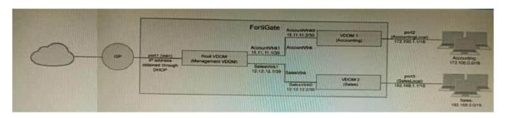
A customer has deployed a FortiGate 300E with virtual domains (VDOMs) enabled in the multi-VDOM mode. There are three VDOMs: Root is for management and internet access, while VDOM 1 and VDOM 2 are used for segregating internal traffic. AccountVInk and SalesVInk are standard VDOM links in Ethernet mode.
