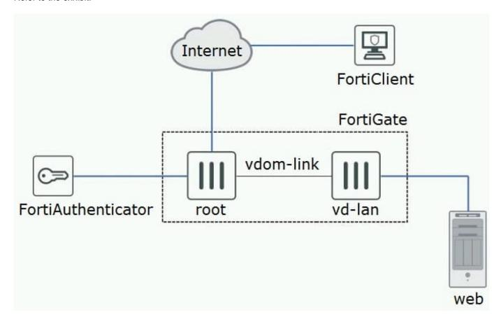
The exhibit shows a topology where a FortiGate is split into two VDOMs, root and vd-lan. The root VDOM provides external SSL-VPN access, where the users are authenticated by a FortiAuthenticator. The vd-lan VDOM provides internal access to a Web server.
