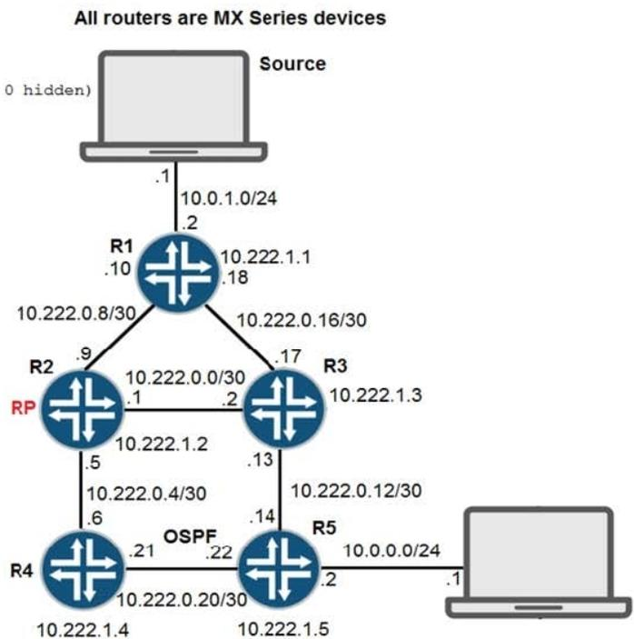
Referring to the exhibit, the source is currently sending multicast traffic using group 224.1.1.1, which is being received by R1. R2 is not receiving PIM register messages.
