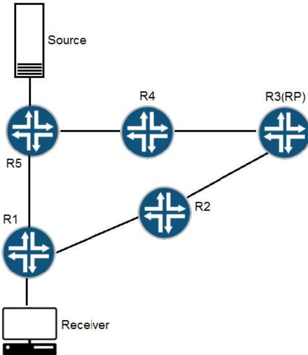
Referring to the exhibit, a PIM-SM network is set up to enable communication between multicast devices. Which statement is true in this scenario?
