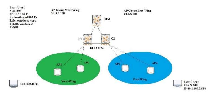
Two Aruba Mobility Controllers (MC) are managed by a Mobility Master (MM) in a non-cluster deployment as shown in the exhibit.
