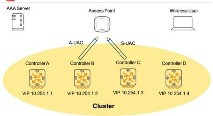
An AP is connected to a cluster of controllers. An AAA server provides all authentication and authorization functions for wireless users. A wireless user connects to an AP, and Active User Anchor Controller (AUAC) and Standby UAC (S-UAC) tunnels are built from the AP to the respective controllers in the cluster.
