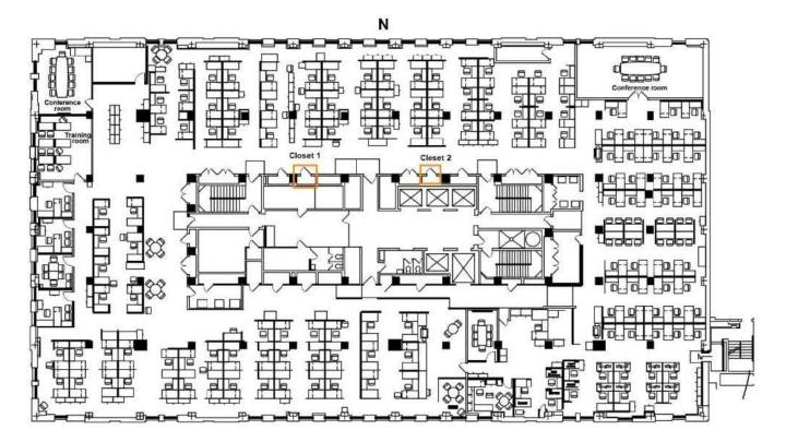
This floor has a central main corridor with washrooms, stairs, elevators and supply, and network cabinets. There are cubicles around the perimeter of the floor. The central part main corridor\\'s dimensions contain 9,350 square feet (870 square meters). The company has determined that Wi-Fi coverage will not include the central area of each floor, which
