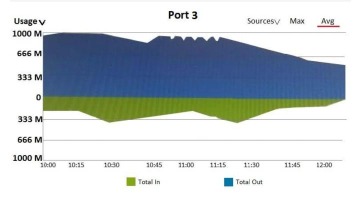
A customer needs a wired network upgrade and has complained about performance issues. The architect has collected information about traffic flow on several switch ports in different locations across the network, and the results are shown in the exhibit. Each of these ports is a 1Gbps port.
