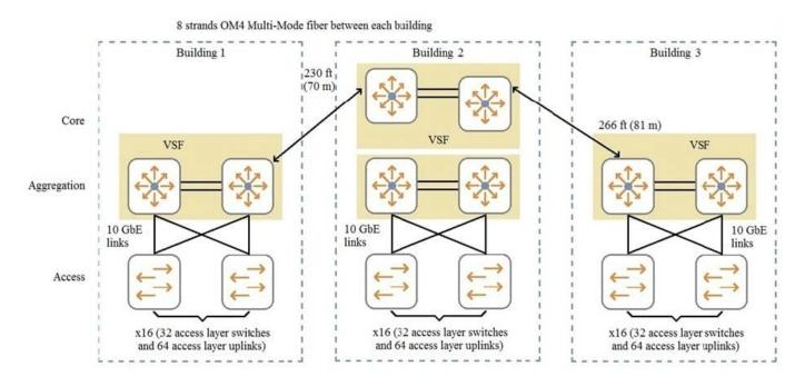
An architect selects 5406R switches for the aggregation layer.
