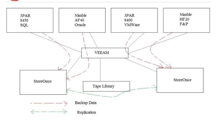
A customer has the environment shown. They currently perform application-consistent daily full backups via Veeam backup to an HPE StoreOnce device. These backups are then replicated to an alternate device using Catalyst copy.
