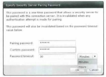
Before you can install a security server, you must configure a security server pairing password. The installation wizard of View Connection Server prompts you for this password.
