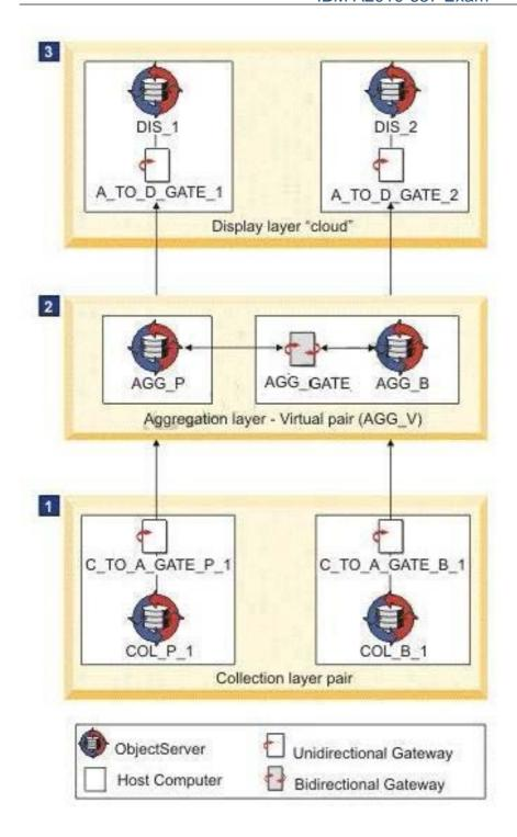
Widgetcom has deployed this 3-tier standard multi-tier architecture deployment of IBM Tivoli Netcool/OMNIbus V7.4 (Netcool/OMNIbus) using the best practice configuration that ships with the product:
