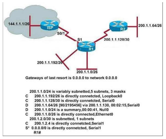
Based on the output of the R1#show ip route command and the information presented in the graphic, which of the following is a potential routing problem?
