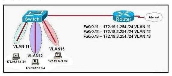
The network shown in the exhibit has just been installed. Host B can access the Internet, but it is unable to ping host C.
