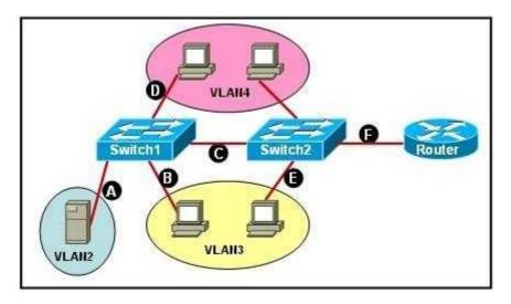
A network associate needs to configure the switches and router in the graphic so that the hosts in VLAN3 and VLAN4 can communicate with the enterprise server in VLAN2.
