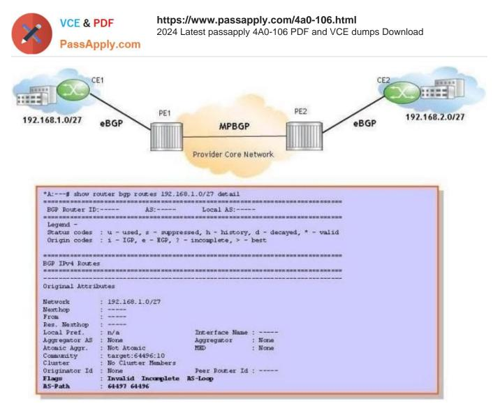
According to the display, a BGP loop is detected for route 192.168.1.0/27. On which router is this command executed?
