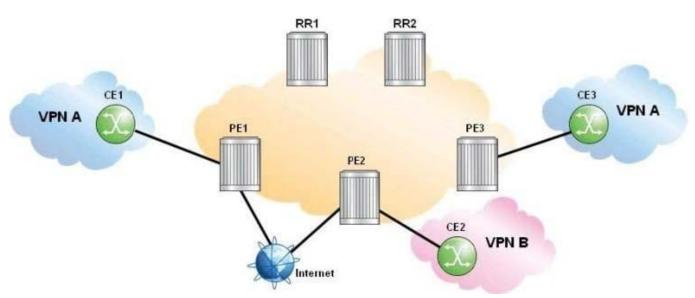
All sites in the displayed network require Internet access. Route reflector 1(RR1) is used for Internet routes only and route reflector 2(RR2) is used for VPN routes only. Which of the following is FALSE?
