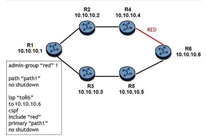
The link between routers R4 and R6 are configured with an admin group "red". What happens when the LSP is first signaled?
