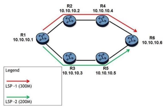
Initially, all links along the path R1-R2-R4-R6 have 400Mbps unreserved bandwidth and all links along the path R1-R3-R5-R6 have 800Mbps unreserved bandwidth. Shared Explicit reservation style is used and Make-Before-Break is enabled. Both fully loose LSPs have been signaled as shown. Later, the configured bandwidth for LSP-1 is changed to 400Mbps. Which of the following is TRUE?
