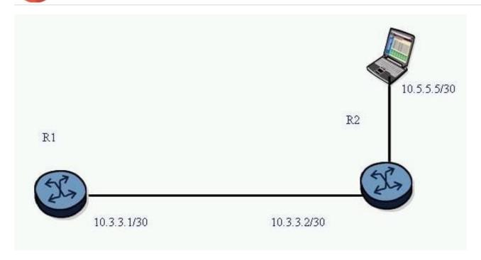
A static route is created on router R1 using the command "static-route 0.0.0.0/0 next-hop 10.3.3.2". What command can be used to test the static route on an Alcatel-Lucent 7750 SR?
