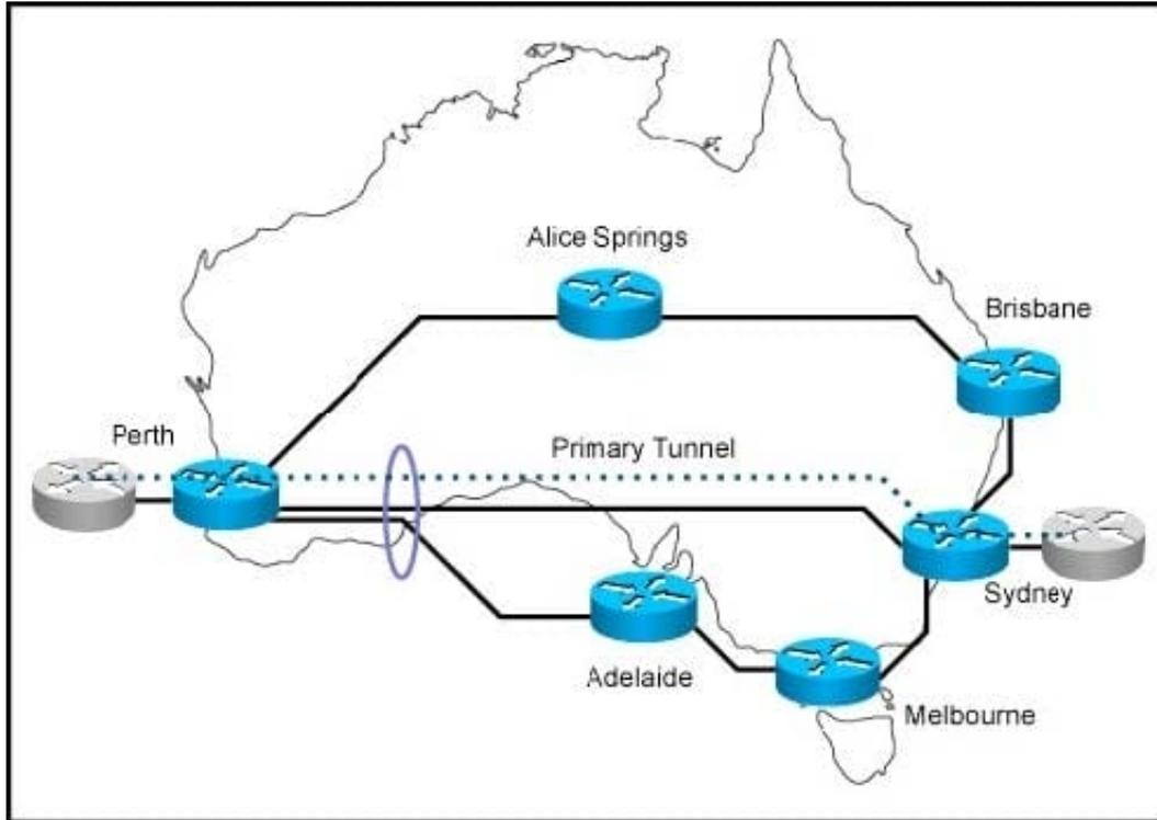
You are designing MPLS-TE for this network. The links from Perth to Sydney and from Perth to Adelaide share the same optical fiber in one given segment. Which feature should you implement to eliminate the risk that a backup tunnel is installed over the same optical fiber as the primary one?
