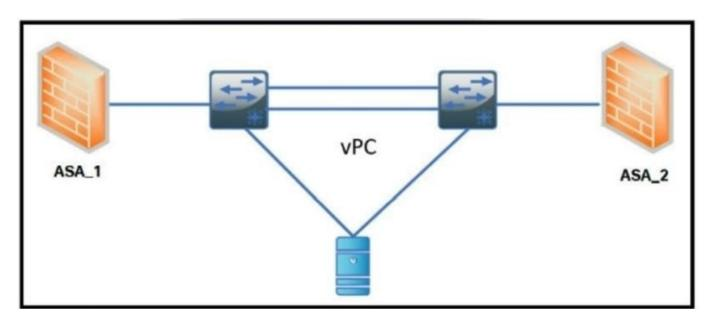
The ASA 1 acts as a Layer 3 gateway for all servers. The servers lose the gateway connectivity when the vPC peer links go down and the vPC keepalive remains up. Which action improves the high availability in the network?
