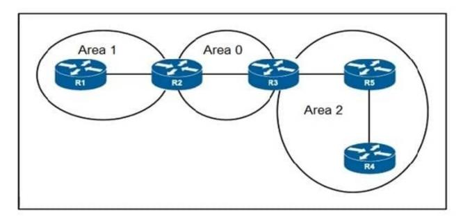
A network engineer applied configuration on R5 to summarize all OSPF routes, but R4 is still receiving specific routes from R5. The engineer has confirmed that both R5 and R4 routers are configured with correct summarization configuration, but R5 is not sending the summary routes. What action must the engineer take to fix the problem?
