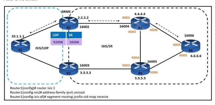
An engineer is configuring service traffic from router R1 to R6 as shown. Which additional configuration must the engineer implement so that the LDP and SR domains will participate and interwork with each other?
