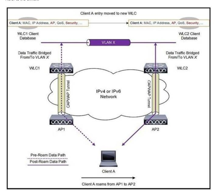
A client roams between two APs that are registered to two different controllers, where each controller has an interface in the client subnet. Both controllers are running AireOS. Which scenario explains the client roaming behavior?
