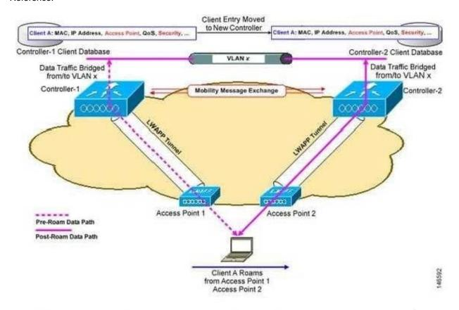
In this instance controllers exchange mobility control messages (over UDP port 16666) and the client database entry is **moved** from the original controller to the new controller.
