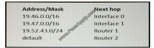
Refer to the exhibit. Which next hop will the router select if given an IP packet with the destination address 19.48.254.3?
