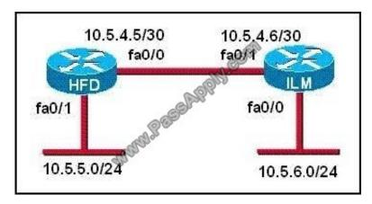
A static route to the 10.5.6.0/24 network is to be configured on the HFD router. Which commands will accomplish this? (Choose two.)
