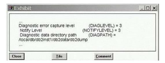
Refer to the GET DB CFG output shown in the exhibit Where can the db2diag.log file be found?
