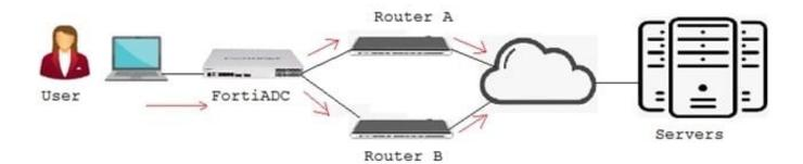
Referring to the exhibit, a FortiADC is load balancing IPv4 traffic between two next-hop routers. The FortiADC does not know the IP addresses of the servers. Also, the FortiADC is doing Layer 7 content inspection and modification.
