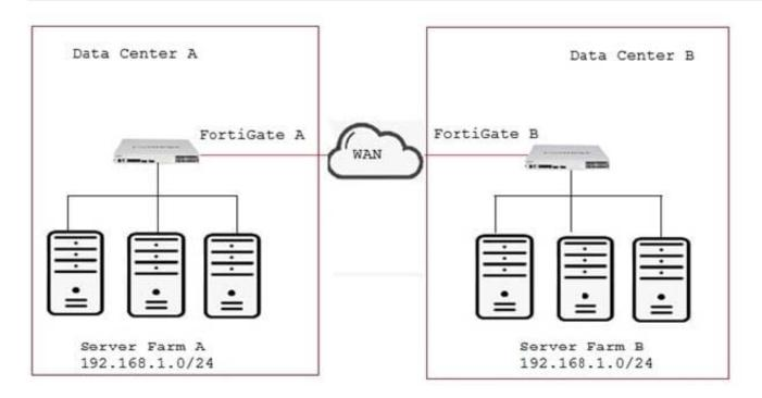
Your company has two data centers (DC) connected using a Layer 3 network. Servers in farm A need to connect to servers in farm B as though they all were in the same Layer 2 segment. What would be configured on the FortiGates on each DC to allow such connectivity?
