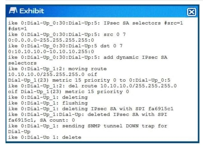
A FortiGate is configured for a dial-up IPsec VPN to allow multiple remote FortiGates to connect to it.
