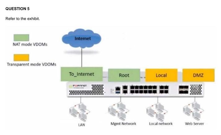
The Root and To\_Internet VDOMs are configured in NAT mode. The DMZ and Local VDOMs are configured in transparent mode.
