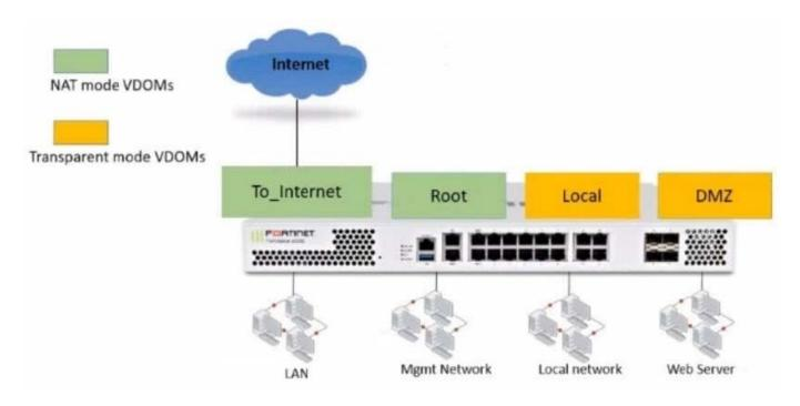
The Root and To\_Internet VDOMs are configured in NAT mode. The DMZ and Local VDOMs are configured in transparent mode.
