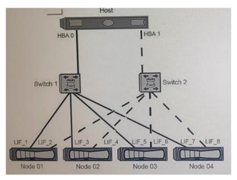
The host in the exhibit is connected to a 4-node ONTAP SAN using dual-fabric implementation. LUNs have been mapped LUN through all available UFs on nil (our nodes. Switch 2 is powered off for high-availability testing. How many paths per LUN would you expect the host to see in this scenario?
