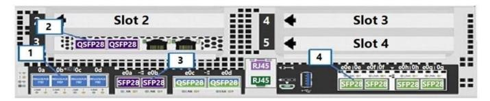
You are installing a 2-node AFF A400 switchless cluster. You have cabled the management network to the e0M port. NetApp also recommends cabling to a redundant management network switch. Referring to the exhibit, to which port should the redundant management network be cabled?
