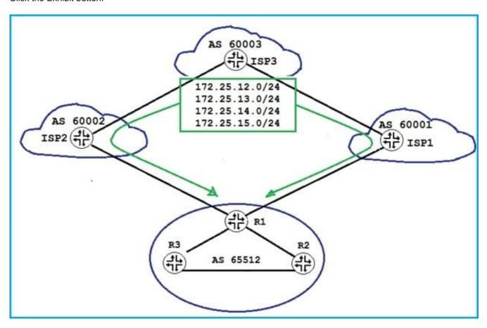
Referring to the exhibit, you have EBGP peerings with both ISP1 and ISP2. You are receiving the 172.25.12.0/24, 172.25.13.0/24, 172.25.14.0/24, and 172.25.15.0/24 routes through both neighbors. You must ensure that traffic to these prefixes are load balanced through both service providers. You have configured a load-balancing policy and have applied it to the forwarding table, but the prefixes are not being load balanced.
