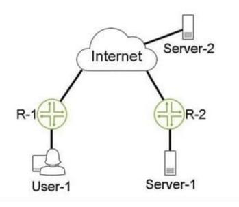
Referring to the exhibit, the GRE tunnel between R-1 and R-2 allows connectivity between User-1 and Server-1. When User-1 communicates with Server-2 with packets that are 1472 bytes in size, no packet fragmentation occurs. User-1 can communicate with Server-1 with packets that are up to 1448 bytes in size with no packet fragmentation. However, if the packet size is larger than 1448 bytes, packet fragmentation occurs.
