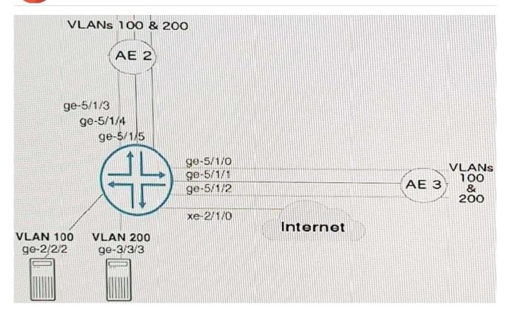
On an MX Series device, you must enable routing between VLANs 100,200, and the Internet ge-5/1/0, and ge-5/1/2 are bundled into interface ae3. Ge-5/1/4, and ge-5/1/5 are bundles into interface ae2. Both AE bundles trunk VLANs 100 and 200. In this scenario, what is the correct configuration snippet for VLAN 100?
