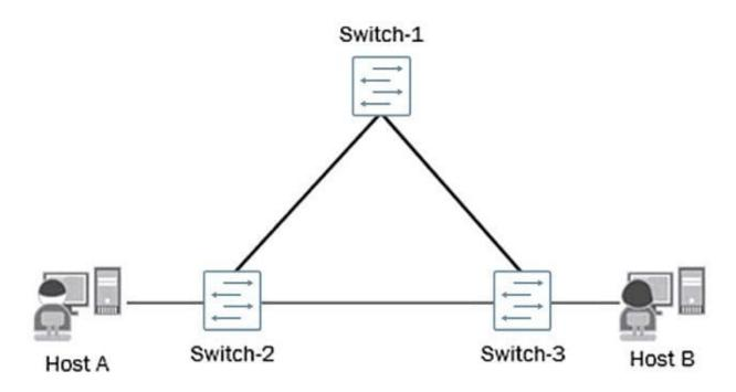
A number of reports from end users indicate that internal and external communications are intermittent and not reliable. You verified the status of the switch ports and have determined that they are up and operational. You also noticed a very high level of link bandwidth utilization on those same ports. The current topology of the affected environment is shown in the exhibit.
