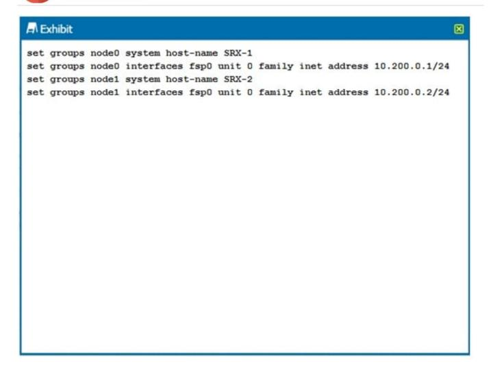
You are configuring an SRX chassis cluster with the node-specific hostname and management address. Referring to the exhibit, which configuration completes this requirement?
