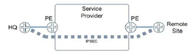
You are asked to design a solution that will provision a circuit from the corporate headquarters to a remote branch. The circuit must be secure, and must support IGP adjacencies. IPsec has been chosen to secure traffic across the WAN connection.
