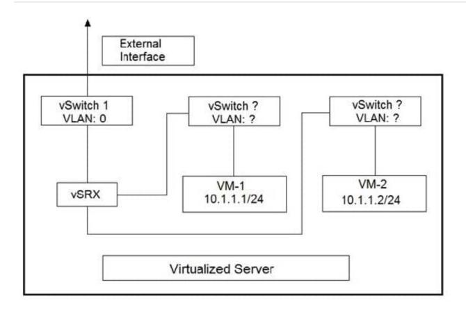
You are designing the virtualized server deployment shown in the exhibit in your data center. The vSRX device is acting as a Layer 2 firewall and the two VMs must communicate through the vSRX device.
