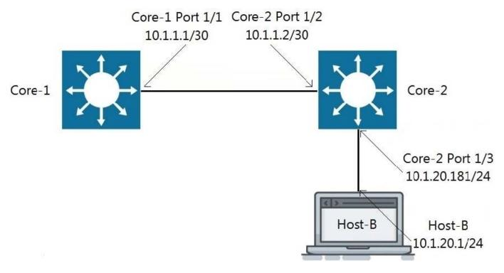
Traffic is failing between Core-1 and Host-B. IP addressing has correctly been applied, and all interfaces are attached to the vrf GREEN.
