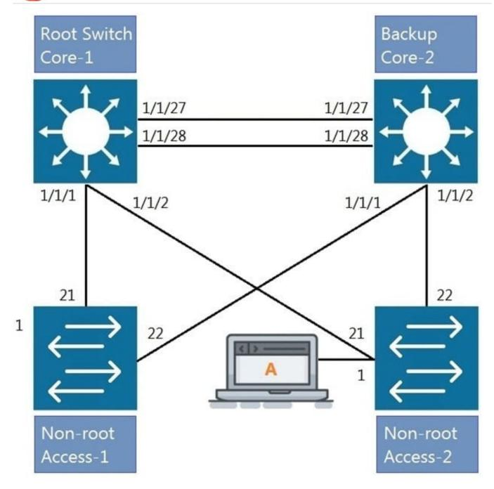
All four switches in the diagram have been configured with the region name "Aruba1".
