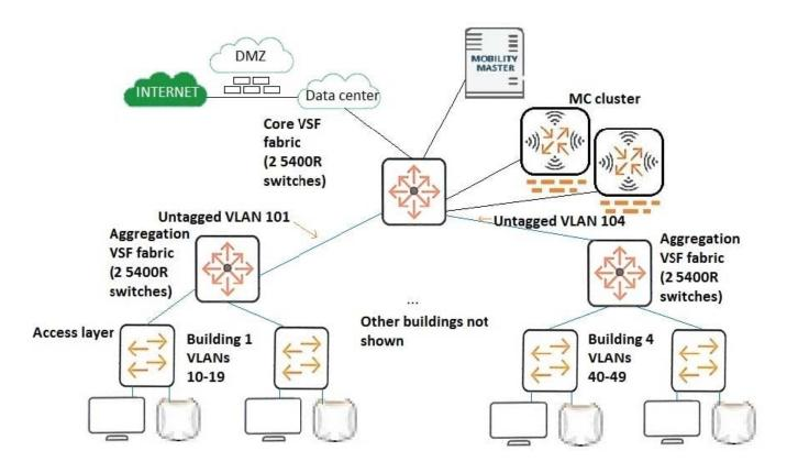
A customer has a wired infrastructure shown in the exhibit. The customer is in the process of expanding their wireless services. They will now add a new wireless solution, with mobility controllers (MCs) connected as shown. The new wireless solution will support a total of 450 APs and about 26,000 wireless devices. It must provide seamless roaming across the entire campus.
