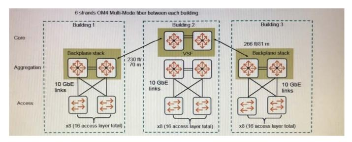
An architect determines that 80 Gbps bandwidth is required for the link aggregation between the Building 1aggregation layer and Building 2.
