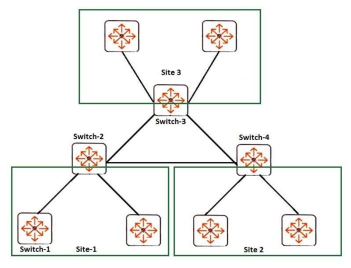
The routing switches shown in the exhibit use OSPF, and all of their interfaces are in Area 1. A faulty link on Switch-1 went up and down many times over the course of several hours. This caused link state updates (LSUs) to flood all of the routing devices in the OSPF AS and reduce performance. The network administrator fixed the faulty link on Switch-1, but the administrator also wants to mitigate the effects if a similar issue occurs in the future.
