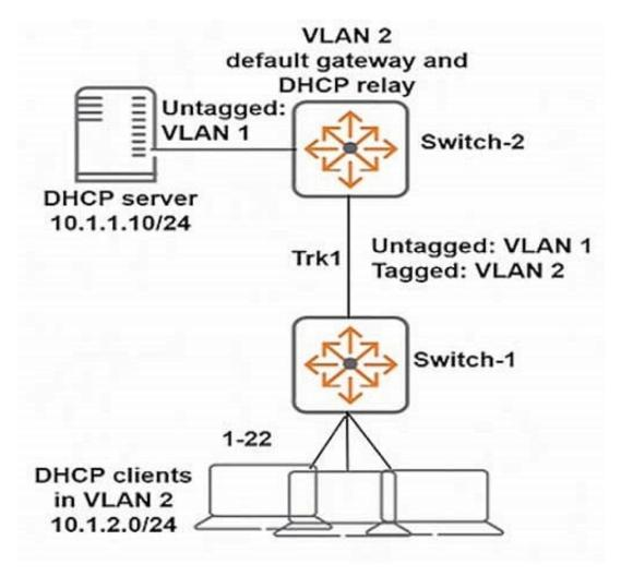
Exhibit 2 Which change to the environment would cause clients to fail to receive DHCP settings?
