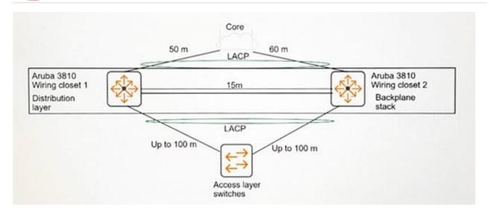
A company requires distribution layer switches that can provide Layer 2 and Layer 3 redundancy. The exhibit shows the proposal for these switches.
