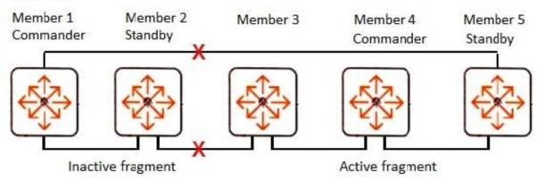
An administrator created a backplane stack with the plug-and-play method and did not after the default backplane stacking settings. Later, who backplane stacking links failed as shown in the exhibit. The network administrator then restored the failed links.
