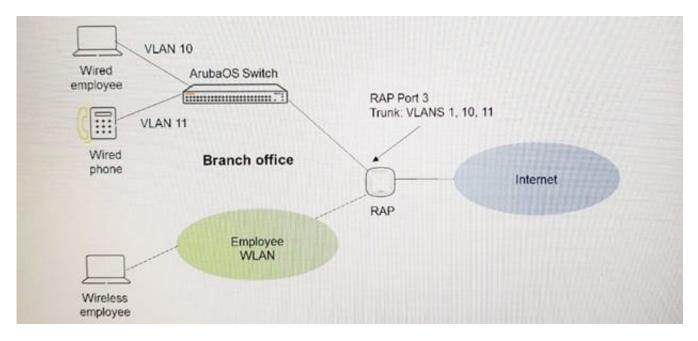
An administrator configures a policy for an AP Group. Port 3 of a RAP is a trunk that connects to a switch at a branch office. VLAN 1 is untagged and VLANs 10 (for data) and 11 (for voice) are tagged. The administrator applies an ACL inbound on Port 3 of the RAP.
