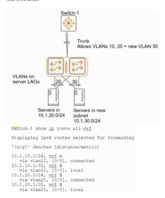
You are adding a VLAN 30, subnet 10.0.30.0/24 to the network shown in the exhibit. (This network is simplified to just the relevant switches for this item.) This subnet belongs in VRF A, and you have added a Layer 3 VLAN 30 interface
