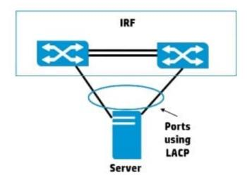
The server shown in the exhibit requires redundant links, and The link aggregation should use LACP. What should the administrator configure on the 1RF virtual switch?
