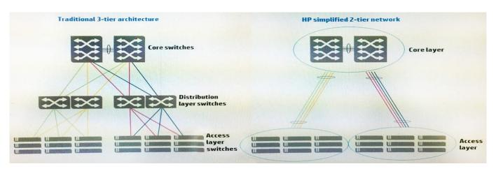
The topology shown on the left of the exhibit illustrates a traditional three-tier architecture. Which technology allows a company to simplify their network with a two-tier topology as illustrated on the right of the exhibit.
