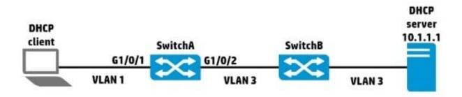
A network administrator needs to configure DHCP on SwitchA. Assume that SwitchA is an HPE Comware switch and is using the default settings for DHCP. The administrator configures the following information:
