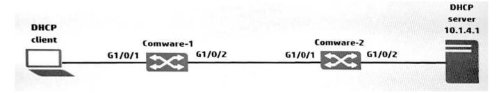
The physical interfaces for Comware-1 and Comware-2 switches in the exhibit are configured in routed mode and OSPF. Both switches have the three subnets in their routing tables. The administrator wants to use DHCP to assign addressing information to the users. Based on the exhibit, where should the administrator configure DHCP relay?
