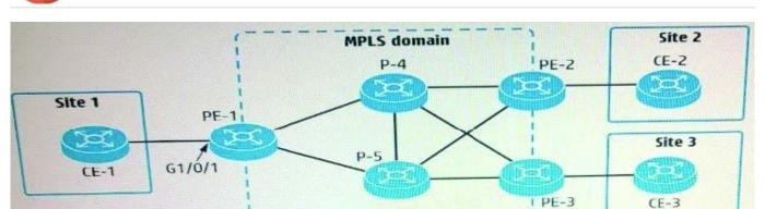
An administrator wants to establish a remote LDP session between PE-1 (loopback IP address 10.0 0.1) and PE-2 (loopback IP address; 10.0.0.2). What is required to do this?
