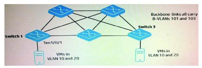
Exhibit 2 The switches shown in the exhibit are implementing SPBM. The administrator is now setting up interface ten1/0/1 to connect to a new VMware host. What is the correct port type and VLAN assignment for the interface?
