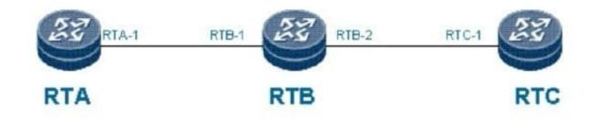
As shown in the figure, RTA connects to RTB and RTC. A TE tunnel is configured on RTA to reach RTC. The TE tunnel cannot be successfully established. However, CSPFbased path calculation is successful and RTA does not receive any PathErro messages. What are possible causes?
