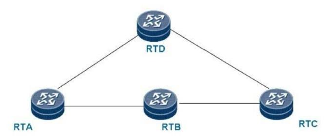
A. When the link between RTA and RTB is faulty, the state of Tunnel1/0/0 is hotstanby inuse.
